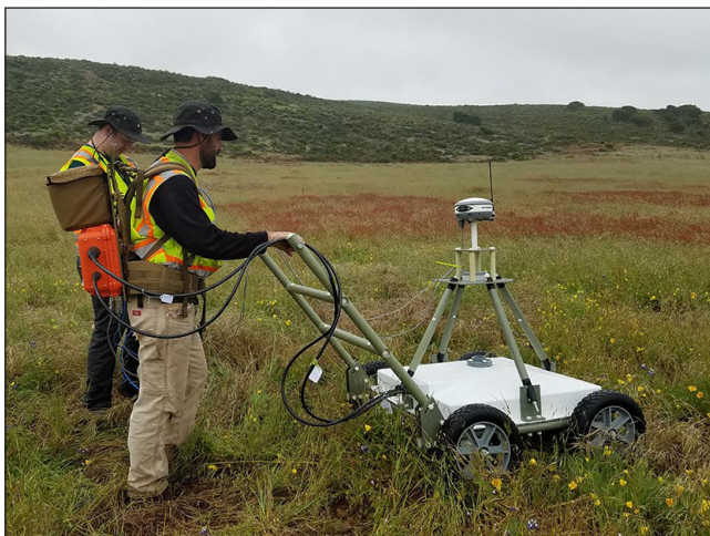
MetalMapper 2x2 static data collection
